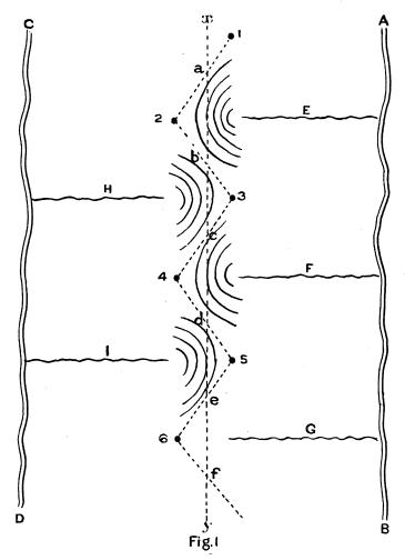
The straight dotted line xy is the axis of original uplift; the zigzag line is the final watershed. AB, CD are main rivers; E, F, G, H, I tributary streams with cirques at their heads. 1, 2, 3, 4, 5, 6 are peaks on crest of main divide; a, b, c, d, e, f are cols between the peaks. The figure is drawn in recollection of a similar diagram in Professor Marr's 'Scientific Study of Scenery.'
