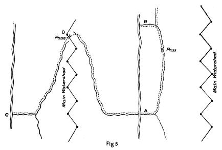
The route from A to C follows the south-flowing streams  $vi\hat{a}$  D. Route from A to B follows the inland valleys higher up the flank of main divide, instead of keeping to main trough.
